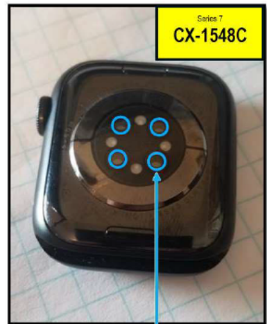
Openings Comprising Opaque Lateral Surface/Opaque Material (Two-Step Opaque PVD Coating + Opaque Ink) Configured to Avoid Light Piping Through the Protrusion
