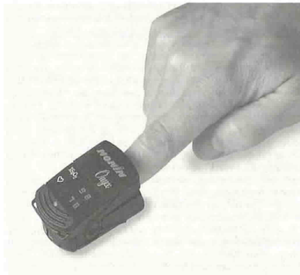
Figure 12.5 A small Nonin model 9500 pulse oximeter designed for emergency evacuation purposes (courtesy of Nonin Medical Inc.).
