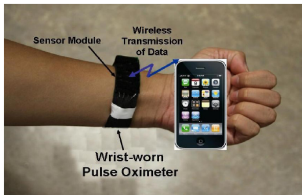
FIGURE 2. Wireless transmission of sensor data from the wrist pulse oximeter.
