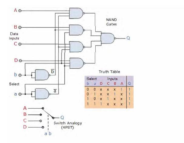
The Boolean expression for this 4-to-1 Multiplexer above with inputs A to D and data select lines a, b is given as:
