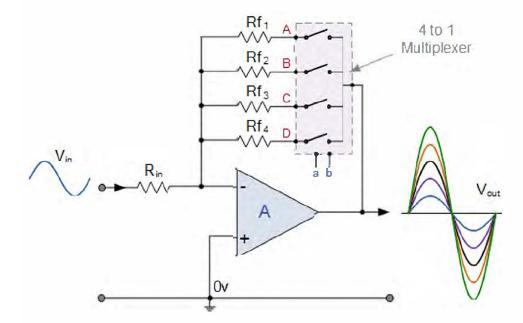
Here, the voltage gain of the inverting operational amplifier is dependent upon the ratio between the input resistor,  $R_{IN}$  and its feedback resistor,  $R_f$  as determined in the Op-amp tutorials.
