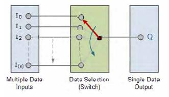
The rotary switch, also called a wafer switch as each layer of the switch is known as a wafer, is a mechanical device whose input is selected by rotating a shaft. In other words, the rotary switch is a manual switch that you can use to select individual
