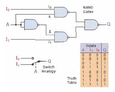
The input A of this simple 2-1 line multiplexer circuit constructed from standard NAND gates acts to control which input  $(I_0 \text{ or } I_1)$  gets passed to the output at Q.
