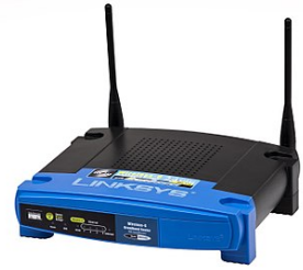
This Linksys WRT54GS , a combined router and Wi-Fi access point, operates using the 802.11g standard in the 2.4 GHz ISM band using signalling rates up to 54 Mbit/s .
