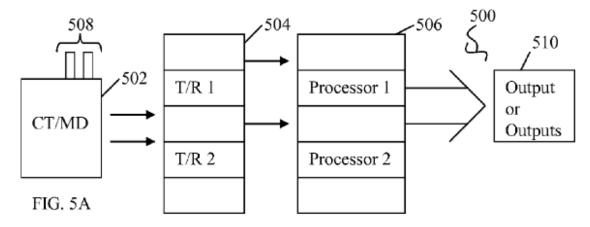
Figure 5A shows a "a dual antenna, dual T/R unit in a CT/MD interfacing with a dual processor." Ex. 1001, 2:15–17. Dual antenna 508 and dual T/R unit 504 interface with dual processor 506 in dual band
