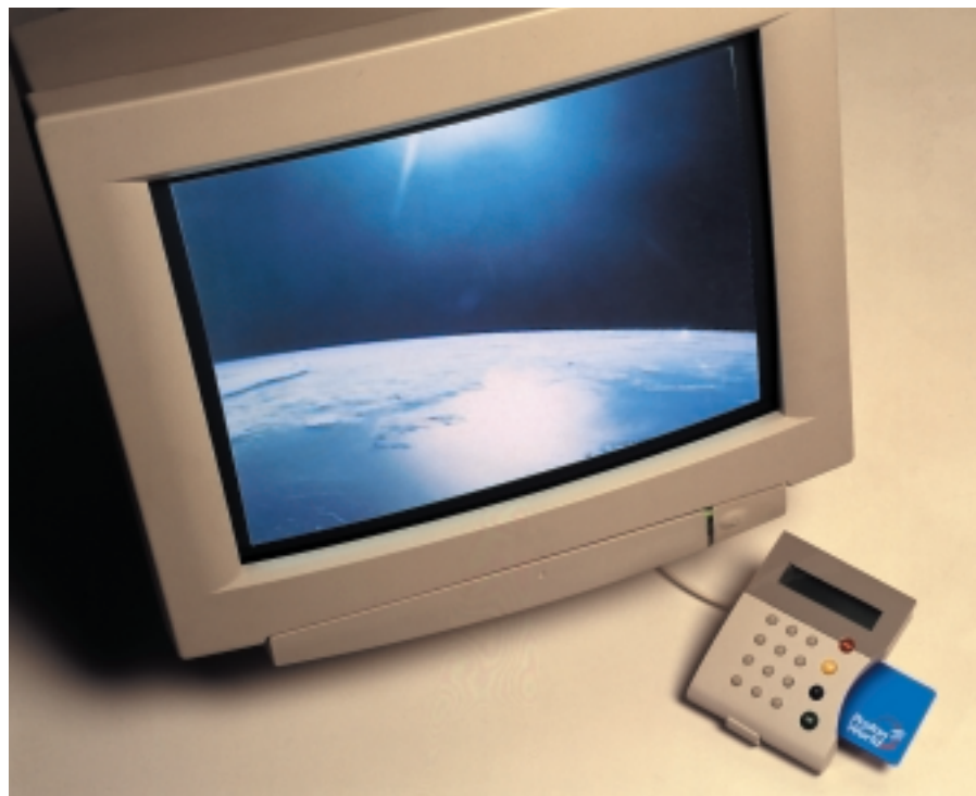
Banksys' C-ZAM/PC: a chip card reader for internet payments and e-purse reloads.
