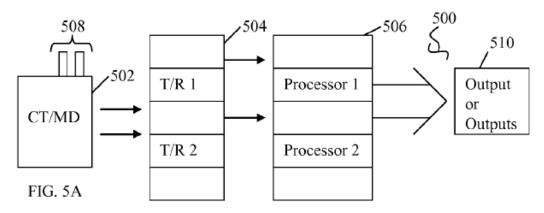
Figure 5A shows a "a dual antenna, dual T/R unit in a CT/MD interfacing with a dual processor." Ex. 1001, 2:15–17. Dual antenna 508 and dual T/R unit 504 interface with dual processor 506 in dual band system 500. *Id.* at 4:37–39. System 500 can communicate through outputs 510, which can be "fibre optic channel, ethernet, cable, telephone, or
