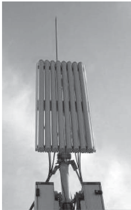
Figure 2.19 Example of a directional beam-forming antenna for a TD-SCDMA system (Photo courtesy of Comba Telecom)
