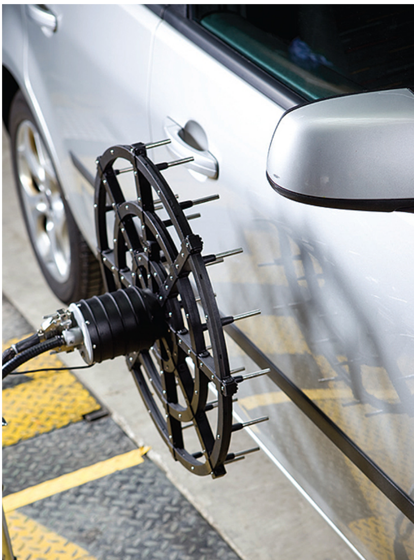
Figure 4: Acoustic arrays featuring many microphones can be used close to a source to accurately capture sound energy in the near field.
