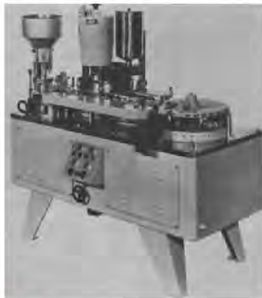
Figure 45-46. MG-2, automatic capsule-filling machine (courtesy, Supermatic).
