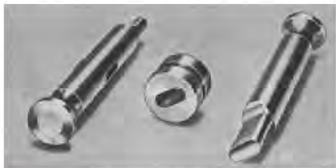
Figure 45-2. Basic mechanical unit for tablet compression: lower punch, die, and upper punch (courtesy, Vector/Colton).
