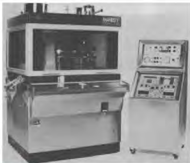
Figure 45-48. Hoeftiger & Karg automatic capsule-filling machine, Model GFK 1200 (courtesy, Amaco).
