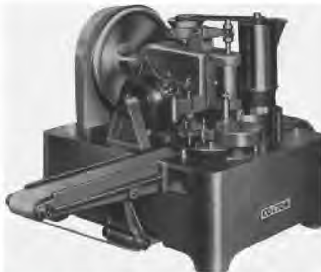
Figure 45-35. Automatic tablet triturate machine (courtesy, Vector-Colton).
