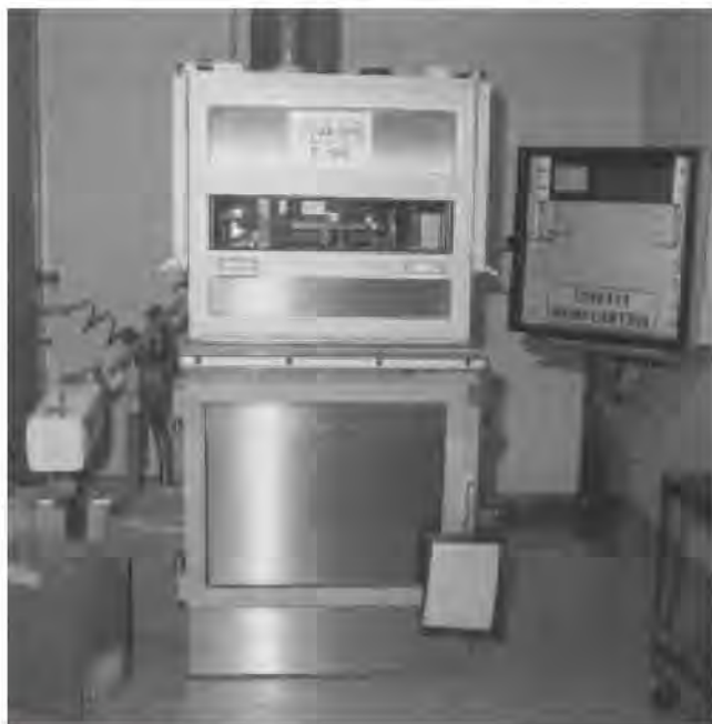
Figure 45-27. Courtoy R-100 with computer-controlled operation.
