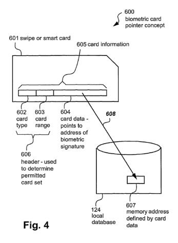
Figure 4, of the '039 patent, above, illustrates swipe or smart card 601 including card information 605 encompassing fields for card type 602, card range 603, and card data 604. The '039 patent describes that "the card data 604 acts as the memory reference which points, as depicted by an arrow 608,
