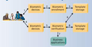
(1) Capture the chosen biometric; (2) process the biometric and extract and enroll the biometric template; (3) store the template in a local repository, a central repository, or a portable token such as a smart card; (4) live-scan the chosen biometric; (5) process the biometric and extract the biometric template; (6) match the scanned biometric template against stored templates; (7) provide a matching score to business applications; (8) record a secure audit trail with respect to system use.
