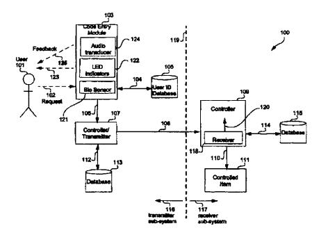
As shown in Figure 2, the major components of the claimed invention are transmitter and receiver subsystems, which work in concert to provide access to a "controlled item." A "controlled
