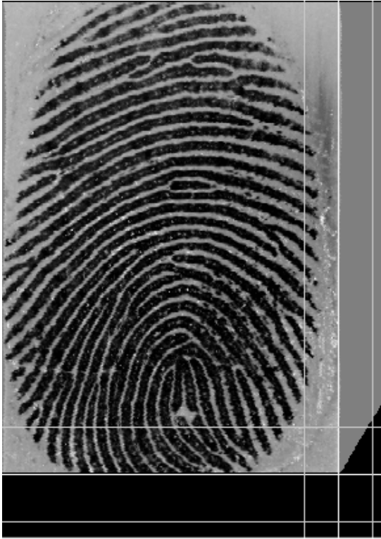
Fig. 8 Result of reconstruction for 0.6 pixels/frame vertical and 0.37 pixels/frame horizontal motion, starting from a smeared image. Grey area on the right is due to padding of the sequence generator, to be able to generate horizontally moving images.
