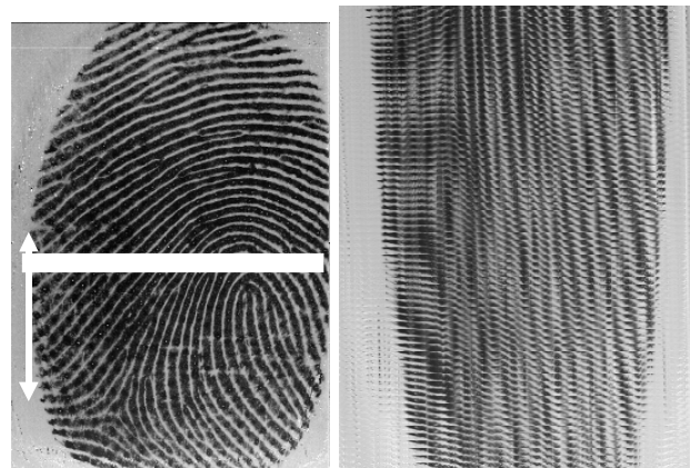
Fig. 2: Example of fingerprint scanning. By simply stacking the sensor output images (on the right), we have an unacceptable result
