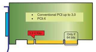
An add-in card complying with any PCI variant can be a 3.3 Volt card.
