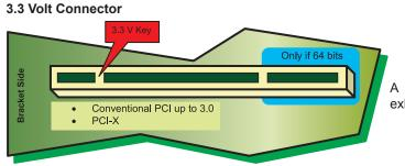
A bus complying with any PCI variant can exhibit the 3.3 Volt connector.
