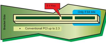
A bus complying with Conventional PCI 3.0 or PCI-X cannot exhibit the 5 Volt connector.
