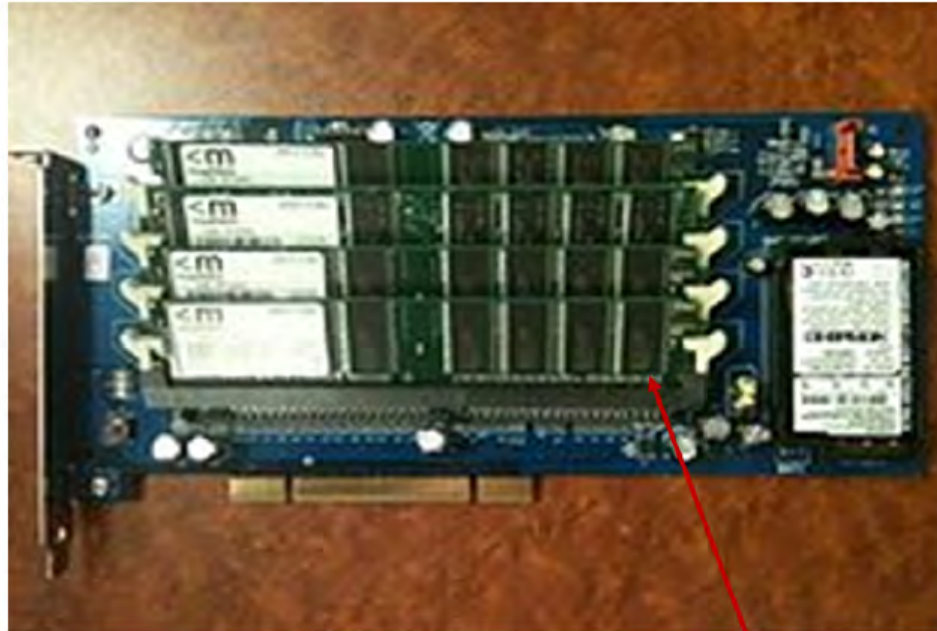
4 slots on PCI populated with 4 DIMMs
