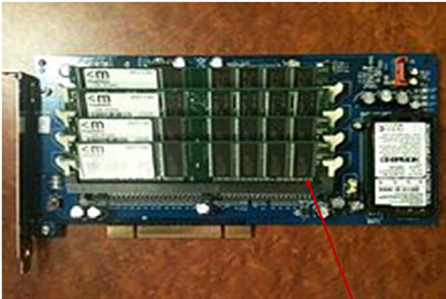
4 slots on PCI populated with 4 DIMMs
