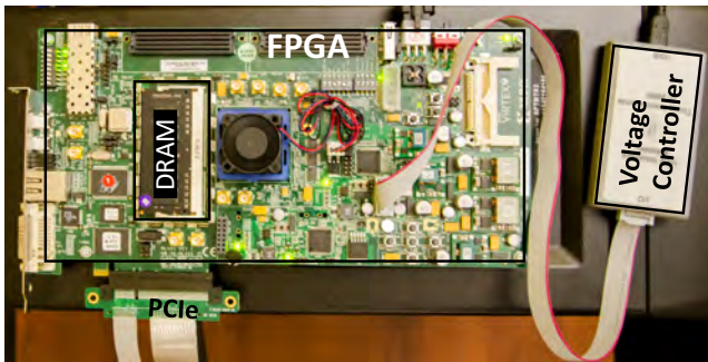
Figure 3: FPGA-based DRAM testing platform.
