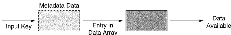
FIGURE Ov.2: An idealized cache lookup. A cache is logically comprised of two elements: the data array and some management information that indicates what is in the data array (labeled “metadata”). Note that the key information may be virtual, i.e., data addresses can be embedded in the software using the cache, in which case there is no explicit key lookup, and only the data array is needed.
