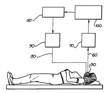
(57) Abstract: An apparatus and a method for the treatment of an upper airway flow limitation, the apparatus including a means to detect an interruption in an upper airway inspiratory flow rate of the patient and further including a treatment means which treats the upper airway flow limitation on detection of the interruption cycle.
