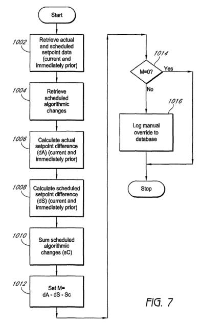
At step 1002 illustrated in Figure 7, a server associated with the thermostat (e.g., a thermostat management server) retrieves setpoint data used to infer the occurrence of a manual override from one or more databases. *Id.* at 3:61–63, 5:55–6:19. At step 1004, the server retrieves any scheduled automated setpoint changes. *Id.* Such changes may include algorithmic changes intended to reduce energy consumption. *Id.*
