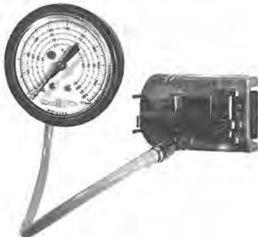
Figure 5.5 Calibration gauge. (Courtesy of Johnson Controls Inc.)
