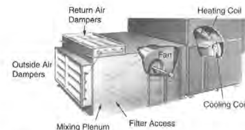
Figure 2.1 Air Handling Unit
