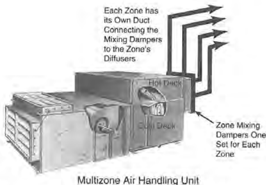
Figure 24.1 Multizone Dampers
