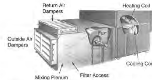
Figure 2.1 Air Handling Unit
