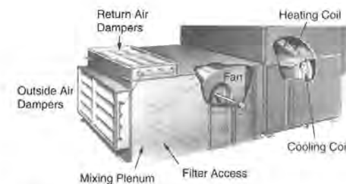
Figure 2.1 Air Handling Unit
