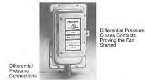
Figure 13.6 Binary Input Status Hardware Point
