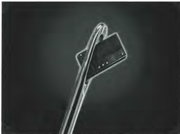
Figure 10.11 Size comparison: low-cost transponder chip in the eye of a needle (reproduced by permission of Philips Electronics N.V.)
