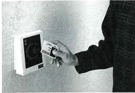
Figure 1.8 RFID reader and contactless smart card in practical use (reproduced by permission of Kaba Benzing GmbH)
