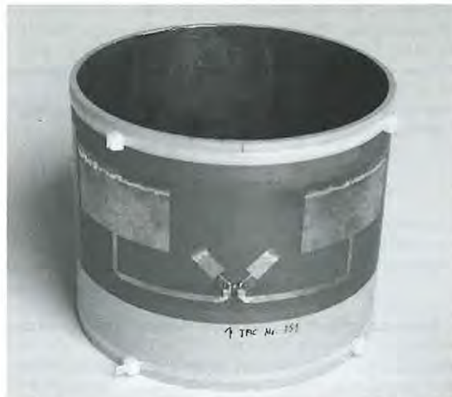
Figure 10.39 Arrangement for measuring the temperature and torque of a drive shaft using surface wave transponders. The antenna of the transponder for the frequency range 2.45 GHz is visible on the picture (reproduced by permission of Siemens AG, ZT KM, Munich)
