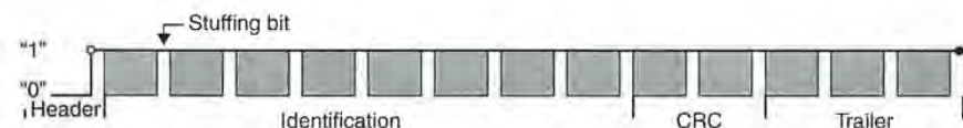
Figure 9.3 Structure of the load modulation data telegram comprising of starting sequence (header), ID code, checksum and trailer
