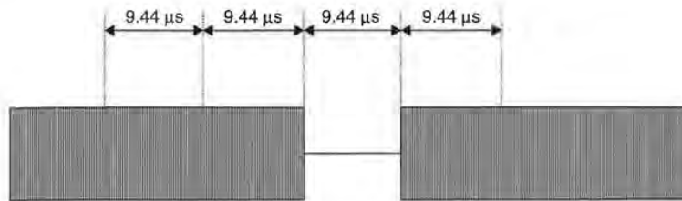
Figure 9.33 The EOF signal consists of a modulation pulse at an even time slot ( t = 2 ) and thus is clearly differentiated from useful data
