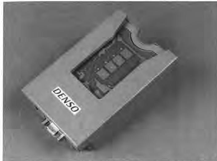
Figure 9.10 Half opened reader for close coupling smart cards in accordance with ISO 10536. In the centre of the insertion slot four capacitive coupling areas can be seen, surrounded by four inductive coupling elements (coils) (reproduced by permission of Denso Corporation, Japan — Aichi-ken)
