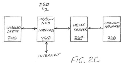
Figure 2C shows a wireless networking scheme. Ex. 1001, 2:1–2. Cellular telephone ("CT") or mobile device ("MD") 202 is in home loop 260 and
