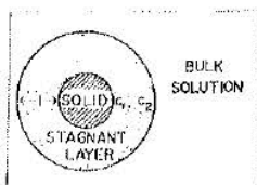
Fig 16-1. Physical model representing the dissolution process.
