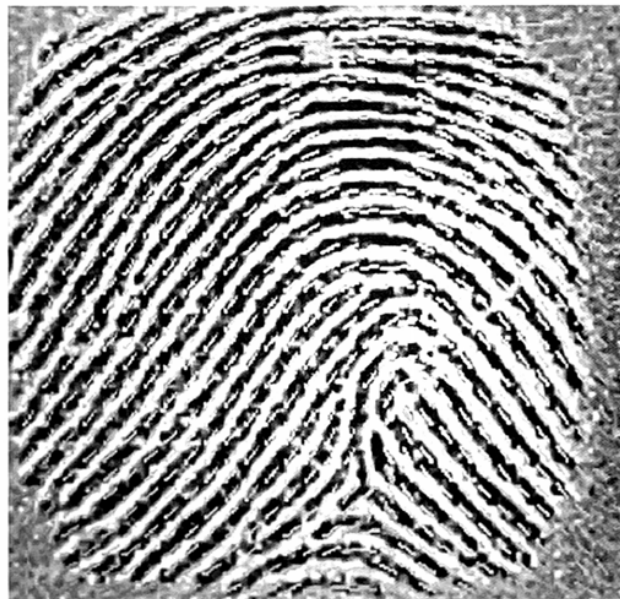
Figure 13.11 Ridge flow vector matrix superimposed on the fingerprint image
