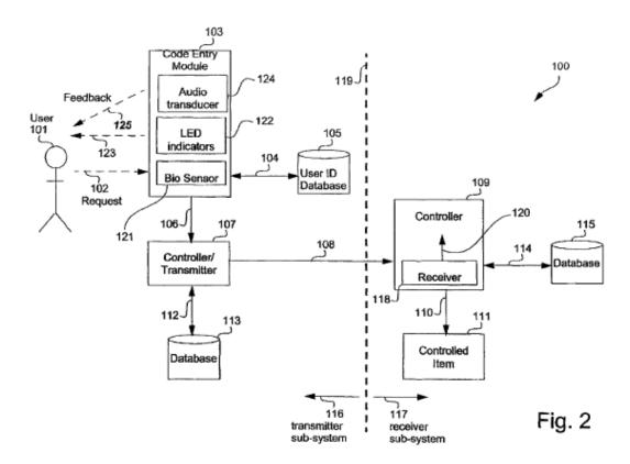
Figure 2 is a functional block diagram of an arrangement for providing secure access according to the system disclosed in the '705 patent. Ex. 1001, 5:18–19.
