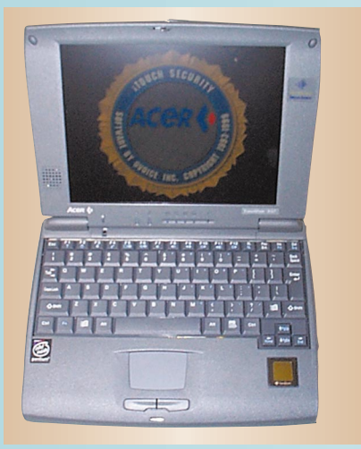
Figure A. Fingerprint authentication devices will find increasing application in securing laptops. The fingerprint sensor is the small rectangle to the bottom right of the keyboard.
