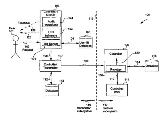
As shown in Figure 2, the major components of the claimed invention are transmitter and receiver subsystems, which work in concert to provide access to a "controlled item." A "controlled item" can be "an electronic key circuit in a personal computer" that is to be accessed by the user. '705 Patent, col. 6, lines 17-20. Representative claim 1 of the '705 Patent reads as follows:
