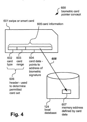
Figure 4, of the '039 patent, above, illustrates swipe or smart card 601 including card information 605 encompassing fields for card type 602, card range 603, and card data 604. The '039 patent describes that "the card data 604 acts as the memory reference which points, as depicted by an arrow 608,
