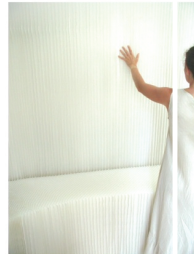
Full-size mock-up of honeycomb structure using tissue paper
