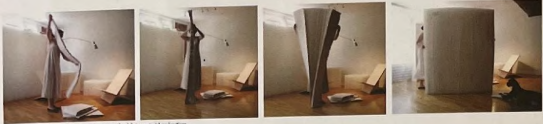
Blankets of honeycomb tissue being opened up into walls - full size material explorations
