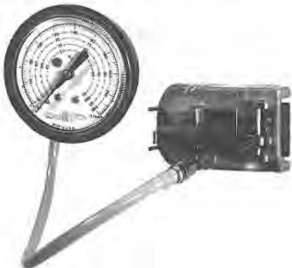
Figure 5.5 Calibration gauge. (Courtesy of Johnson Controls Inc.)
