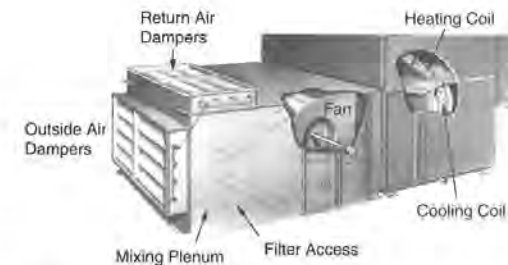
Figure 2.1 Air Handling Unit
