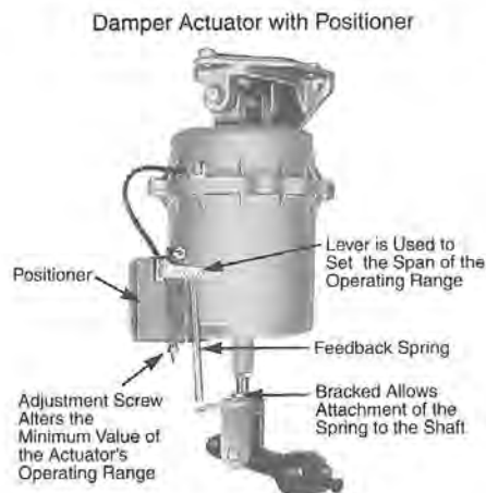
Figure 10.3 Positioning Relay and Damper Actuator
