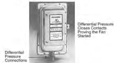
Figure 13.6 Binary Input Status Hardware Point
