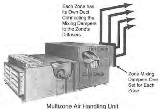
Figure 24.1 Multizone Dampers
