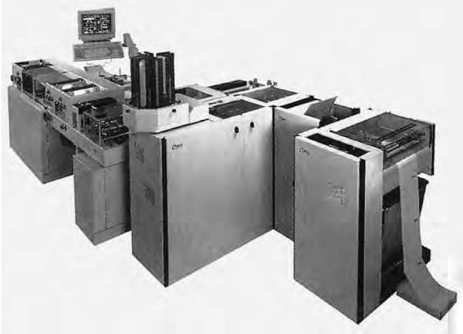
Figure 10.67 A system for attaching cards to their associated letters, which are then stuffed into envelopes along with any necessary attachments. This machine can prepare and stuff up to 7000 envelopes per hour (Source: Böwe Systec)
