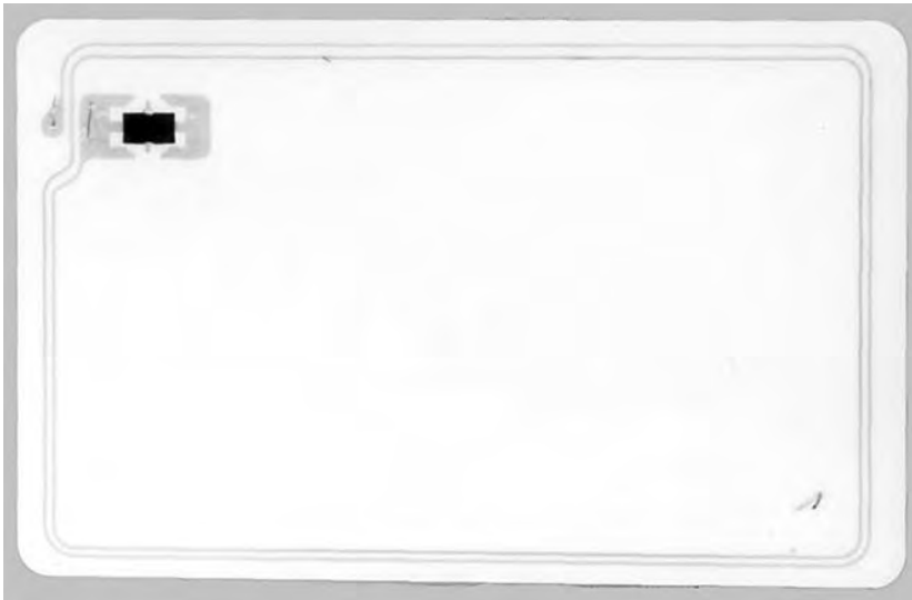
Figure 10.43 Printed coil for a contactless smart card
