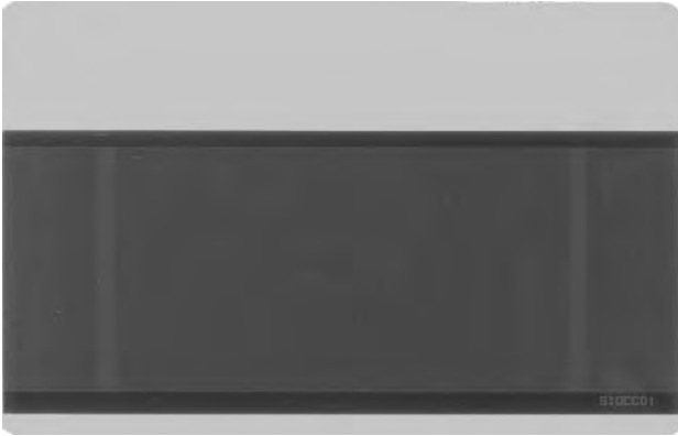
Figure 2.12 A typical optical memory card with a net storage capacity (with error correction) of approximately 4 MB. The raw capacity (without error correction) is approximately 6 MB
