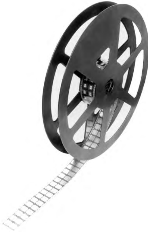
Figure 10.53 A reel with a partial roll of tape carrying paired modules. This is the typical manner in which modules are supplied to the smart card manufacturer by the module manufacturer
