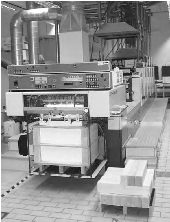
Figure 10.25 An offset printing machine for sheet printing
