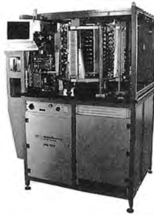
Figure 10.57 An initialization machine that can process 40 cards in parallel ( Source: Mühlbauer)
