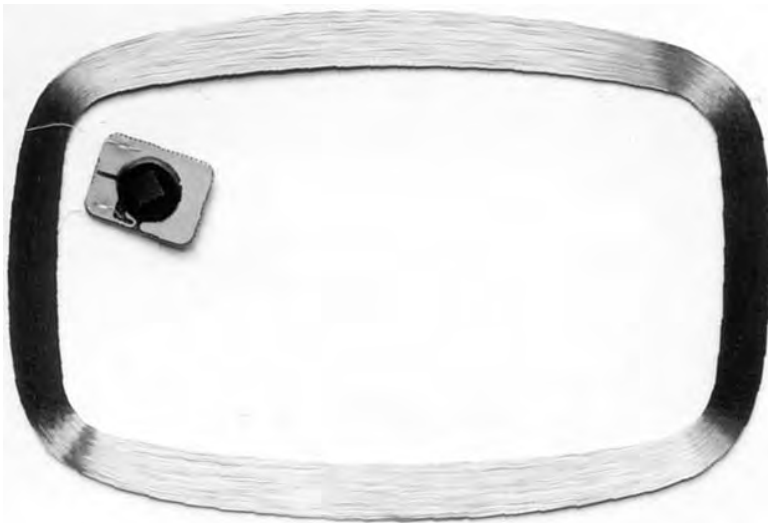
Figure 10.40 A wound coil made from copper wire together with a module, for use in a contactless smart card. This method is now obsolete, but the photo clearly shows the construction of the coil and the module
