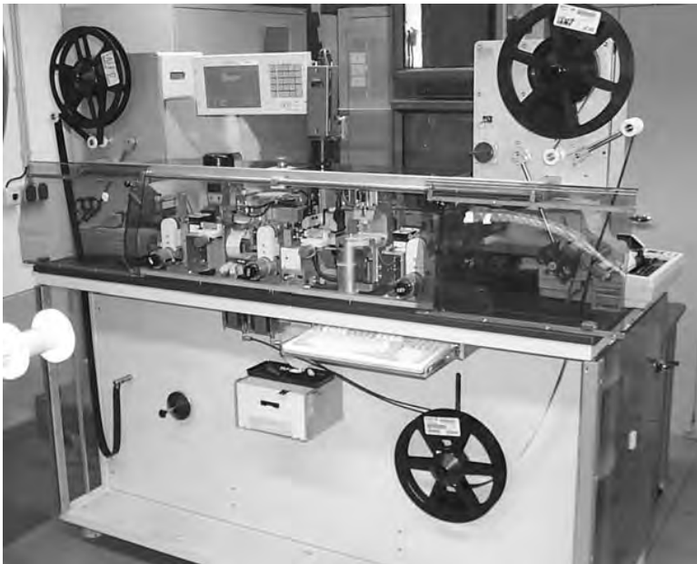
Figure 10.18 An incoming product inspection machine for tape-mounted modules (COT)
