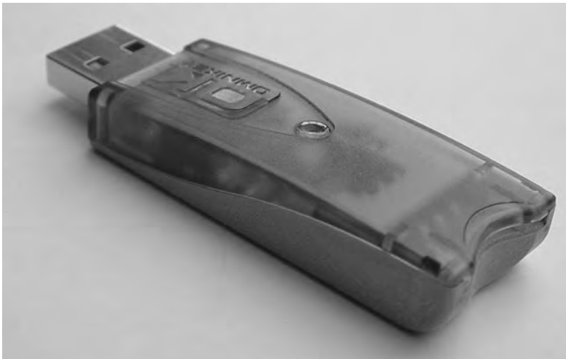
Figure 11.5 A smart card terminal in the form of a USB plug, for use with cards in the ID-000 (plug-in) format
