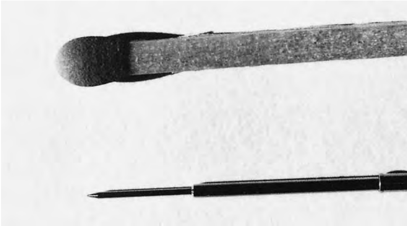
Figure 10.55 Detail view of a probe needle for the contact unit of a high-performance smart card testing station. Although the shape of the probe needle does not conform to the ISO/IEC 7816-2 standard, this type of contact element is often used in production facilities due to its reliability
