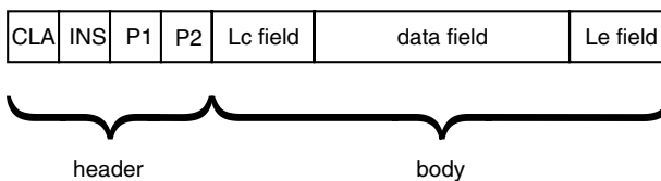
Figure 6.39 Structure of a command APDU
