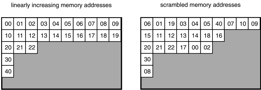
Figure 8.25 Comparison of a conventional semiconductor memory and a scrambled memory used in a smart card microcontroller
