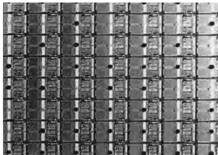
Figure 10.11 Portion of a wafer with microcontroller ICs. The dots on top of some of the chips mark defective devices
