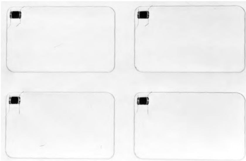
Figure 10.42 Coils for contactless smart cards made using the embedded coil technique, located on a multiple-copy sheet
