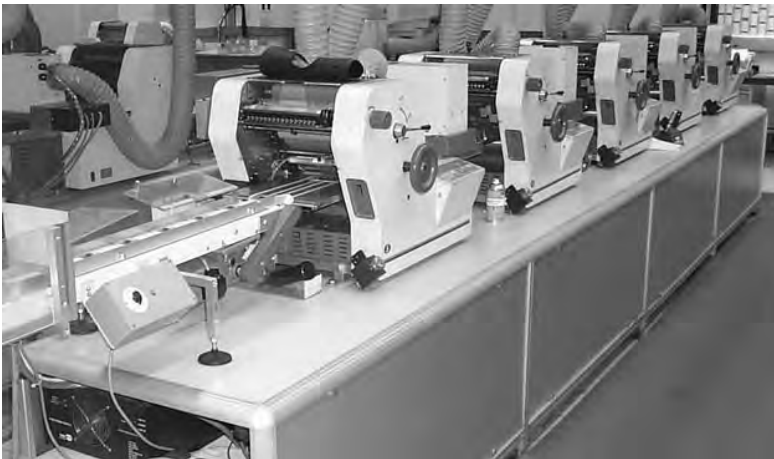
Figure 10.28 Five single-card silkscreen printing machines arranged in series
