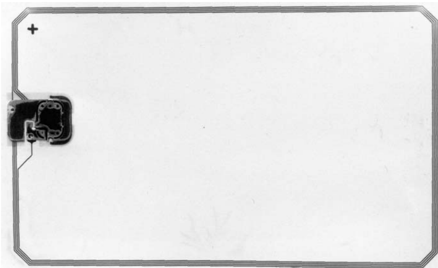
Figure 3.71 Inlay foil for a contactless smart card with inductive coupling using an etched coil
