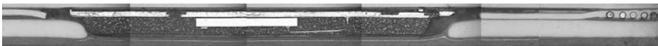
Figure 10.32 Cross-section of a contactless smart card with a module and a wound coil embedded in the card body. The visible edge of the chip inside the module is 2 mm long (Source: Giesecke & Devrient)
