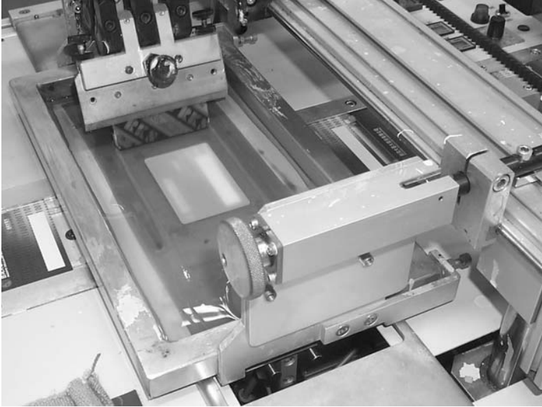
Figure 10.29 Detail of a single-card silkscreen printing machine
