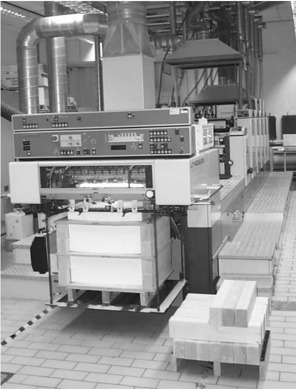
Figure 10.25 An offset printing machine for sheet printing
