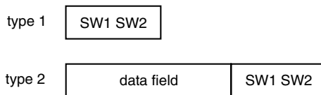
Figure 6.43 The two types of response APDUs
