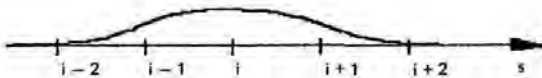
Fig. 8.10 Uniform B-spline: B_i(s) . Its support is non-zero only for s between i - 2 and i + 2 .
