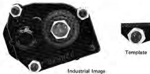
Fig. 3.3 An industrial image and template for a hexagonal nut.
