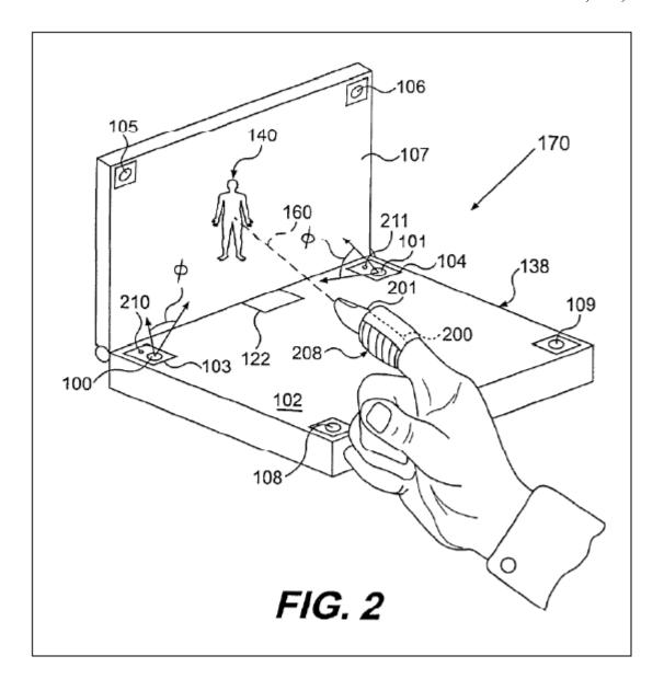
*Id.* at Fig. 2. As illustrated, a laptop 138 may include camera locations 100, 101, 105, 106, 108, 109; keyboard surface 102; screen housing 107; light 122; light emitting diodes (LEDs) 210 and 211, and work volume area 170 within which a user's movements are detected. *Id.* at 2:39-53. The system can detect a user's finger alone or the user may employ external objects such as ring 208 to help detect and recognize gestures performed in work volume area 170. *Id.* at 2:54-3:8. The '079 Patent
