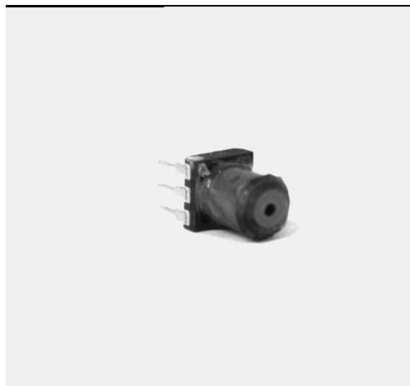
Figure 2.2: The fixed field of view camera. It consists of a four element lens assembly attached directly to a CCD sensor.
