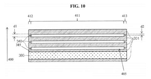
Figure 10 shows a wireless power receiver, which includes printed circuit board 301, short-range communication antenna 340, a receiving coil (not shown), and shielding unit 380. Ex. 1001, 3:4–6, 8:21–23, 8:44–50. Printed circuit board 301 includes multiple layers where each layer is spaced apart
