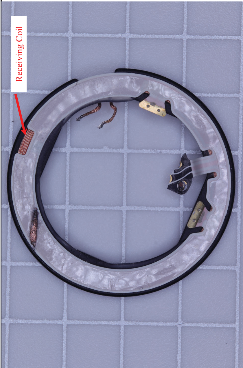
Optical image of the wireless receiving coil from the exemplary Apple Watch Series 6.
