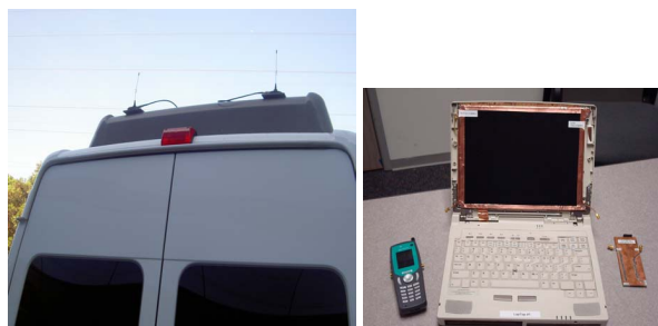
Figure 1. a) AT Antennas mounted on the van roof b) Form factor accurate AT antennas
