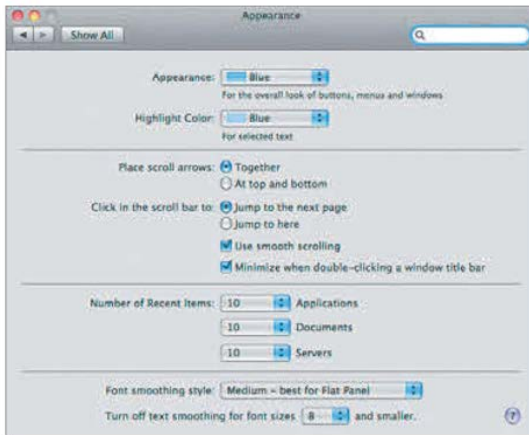
Figure 3.11 You can change Mac OS X's scrolling behavior in the Appearance preference pane.
