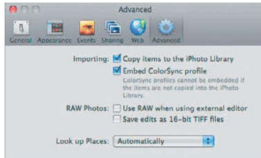
Figure 2.19 Uncheck Copy Items to the iPhoto Library to leave photos imported from your hard disk in their original locations.
